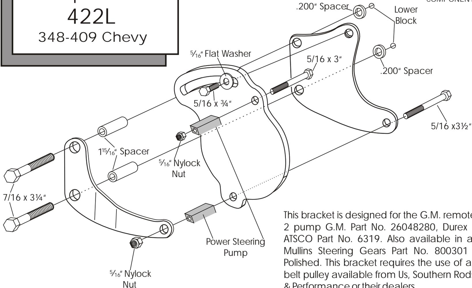
This bracket is designed for the G.M. remote reservoir type 2 pump G.M. Part No. 26048280, Durex Part No. 6319, ATSCO Part No. 6319. Also available in aluminum from Mullins Steering Gears Part No. 800301 Plain, 800302 Polished. This bracket requires the use of an aluminum V-belt pulley available from Us, Southern Rods & Parts, Street & Performance or their dealers.
