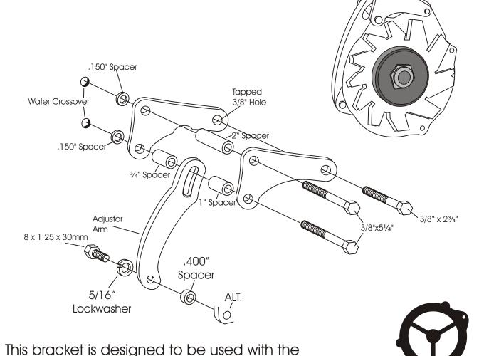
small CS 130 G.M. Alternators with the threaded mounting ear in the 2 o' clock position.
