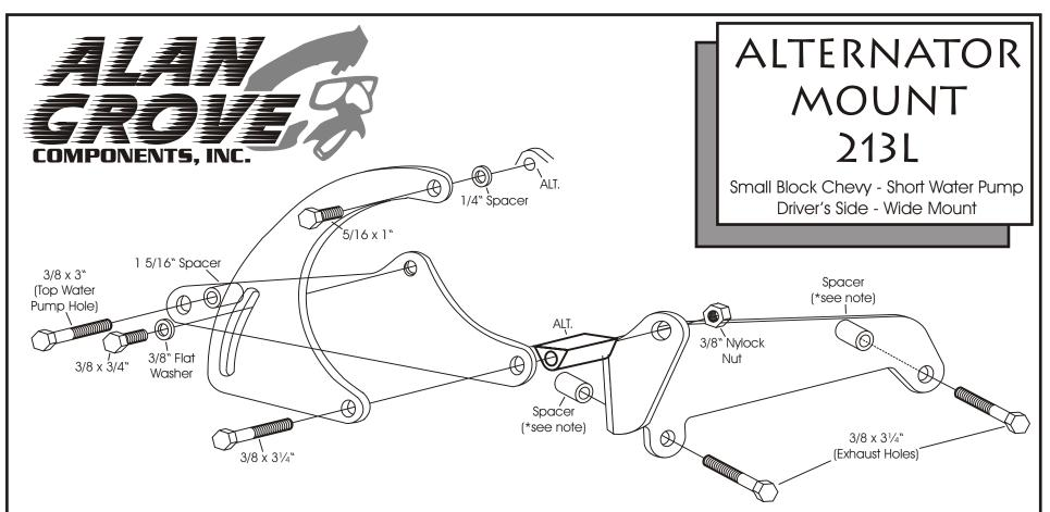
We use a belt length of 57-58" with this mount on installations in our shop. However; this can vary with the diameter of your pulleys.
