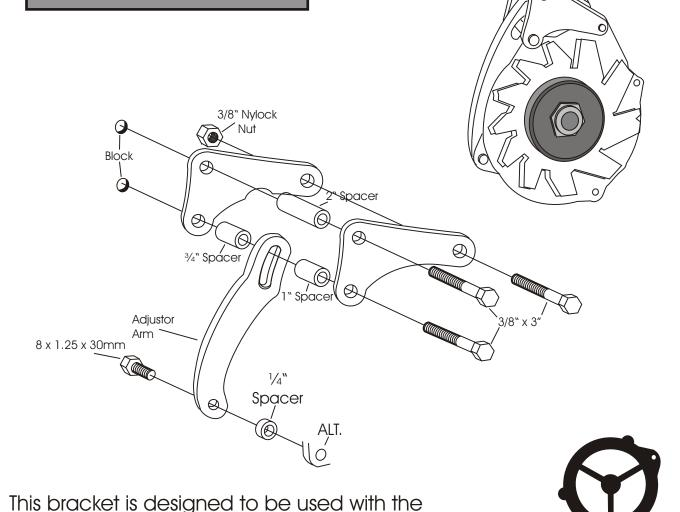
(We use a belt length of 42 to  $42\frac{1}{2}$ " with this mount on installations in our shop. However; this can vary with the diameter of your pulleys.)
