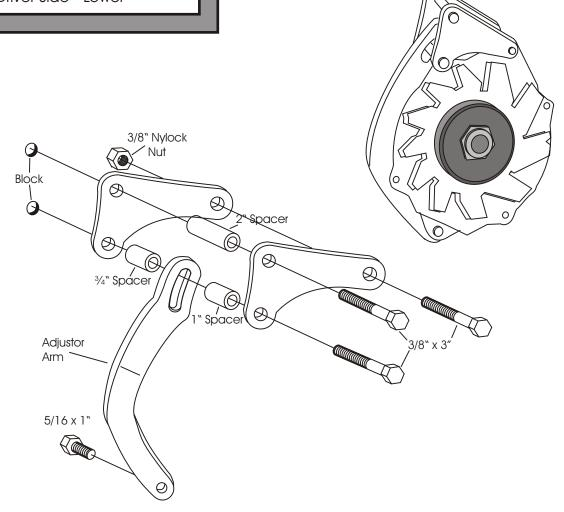
(We use a belt length of  $42\frac{1}{2}$  to  $43\frac{1}{2}$ " with this mount on installations in our shop. However; this can vary with the diameter of your pulleys.)
