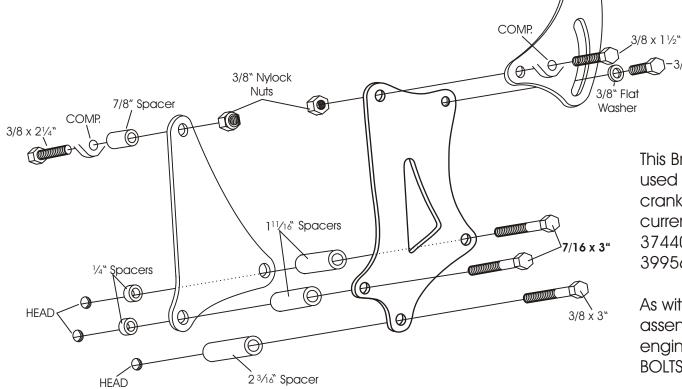
This Bracket was designed to be used with Chevrolet double groove crank and water pump pulleys. The current G.M. Part Numbers are 3744043 for the crank and 3995642 for the water pump.
