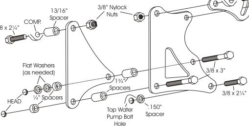
We use a belt length of  $57\frac{1}{2}$  -  $58\frac{1}{2}$ " with this mount on installations in our shop. However; this can vary with the diameter of your pulleys.
