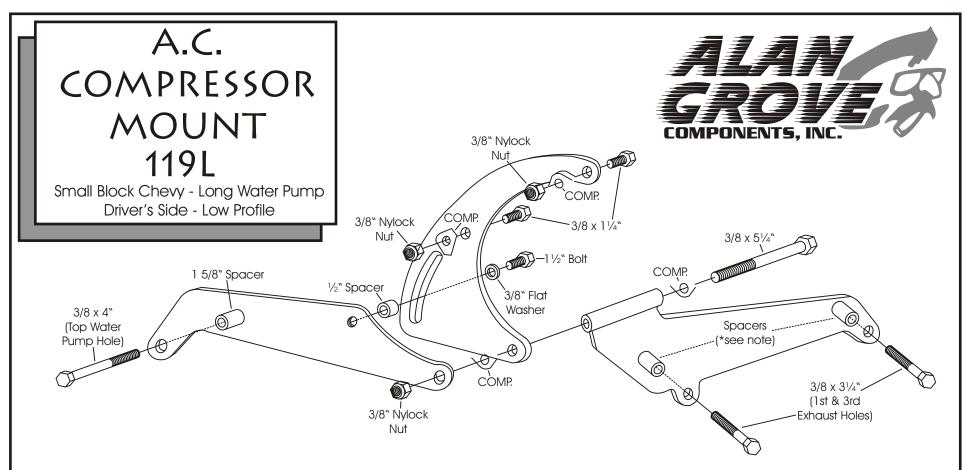
We use a belt length of 60-61" with this mount on installations in our shop. However; this can vary with the diameter of your pulleys.
