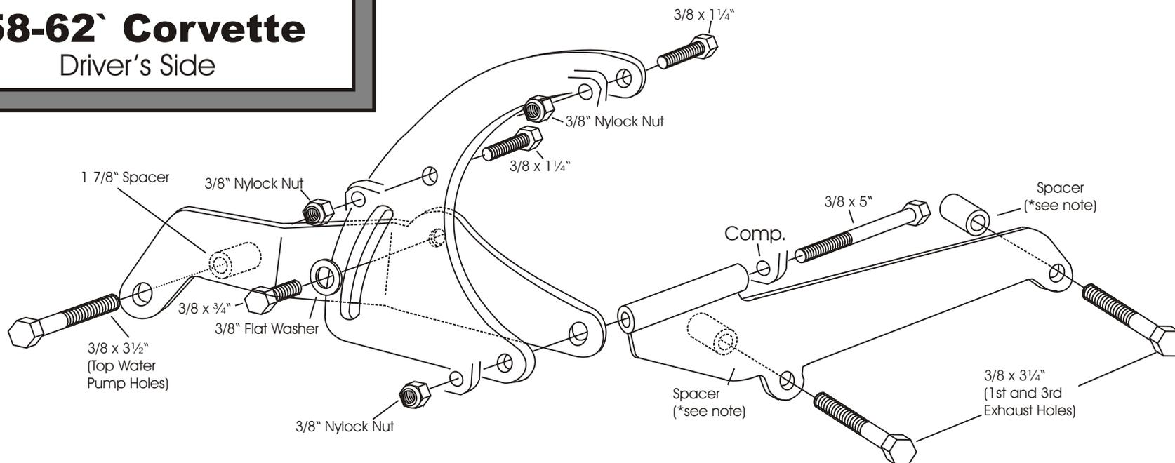
\*NOTE: Exhaust Spacers- with HEADERS- use the 2 1/4" long x 5/8" O. D. Spacers. With RAMS HORN MANIFOLDS use the 1/4" long x 3/4" O. D. Spacer at rear hole of bracket and a 1 1/16" long x 3/4" O. D. Spacer at front hole of bracket. With the later DROP-TYPE manifolds use the 1 1/16" long x 3/4" O. D. spacers at both bracket holes. As with any mount system, assemble all of the brackets to engine BEFORE TIGHTENING THE BOLTS.
