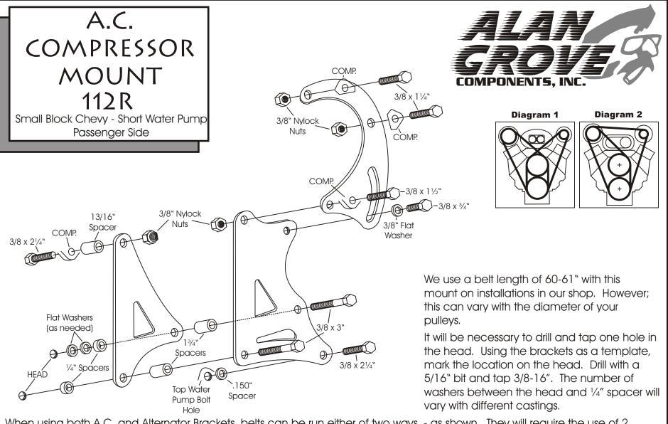
When using both A.C. and Alternator Brackets, belts can be run either of two ways, - as shown. They will require the use of 2 groove crank and water pump pulleys. Routing the belts as shown in Diagram 2 - will allow clearance for small blowers and extra room for T.P.I. air cleaners. The long belt will be approximately 71-72."
